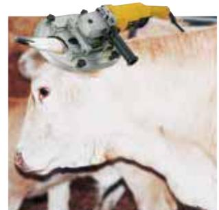
**DESCORNADOR ELÉCTRICO A RED 230 V. MANGO DE PLÁSTICO, TEMPERATURA 620° C. (INCLUYE CABEZAL)**
